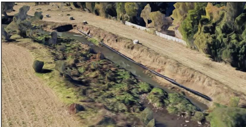
About 90 metres of exposed and sagging pipeline can be seen on the east bank of the Moreleta. The sedimentation in the river bed forced the stream towards the bank which was further weakened by a storm water outlet above the pipe.
